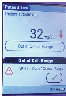
Figure 2. Accu-Chek Inform II glucometer displays the blood glucose as a numeric value, which is the expected format, along with an alarm code of W-511 Out of Critical Range (source of photo: VHA 8 ).
