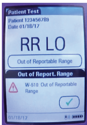
Figure 1. Accu-Chek Inform II glucometer displays the blood glucose with an abbreviation, RR LO (out of reportable range; low limit) and an alarm code, W-510 Out of Reportable Range, below the abbreviation. The “510” in the alarm code has been mistaken as the blood glucose value, leading to incorrect administration of insulin (source of photo: VHA 8 ).
