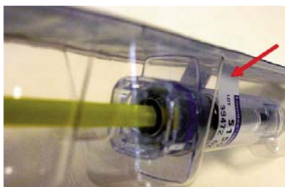
Figure 1. Example of syringe label with edges that no longer adhere to syringe.
