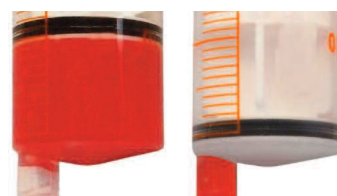
Figure 11. Medication drawn into a syringe using an ENFit adapter but given by mouth leads to under-delivery of medication. The volume of medication in the tip of the syringe differs before and after administration. The dose minus the drug leftover in the dead space was administered.
