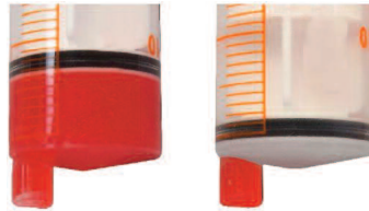
Figure 8. Medication drawn up from a cup without an ENFit connector and delivered by mouth. The volume of medication in the syringe tip at the start and end of administration is the same , so dosing is accurate.
