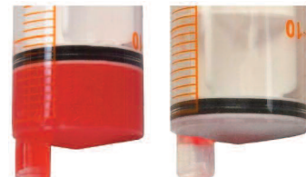
Figure 10. Medication drawn from a cup but administered into an ENFit device can lead to over-delivery of medication. The volume of medication in the tip of the syringe differs before and after administration. The full dose plus the extra in the dead space was administered.
