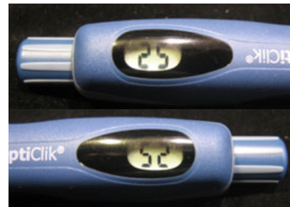
Figure 2. Opticlik injector: Dose of 52 units appears as 25 units if held upside down.
